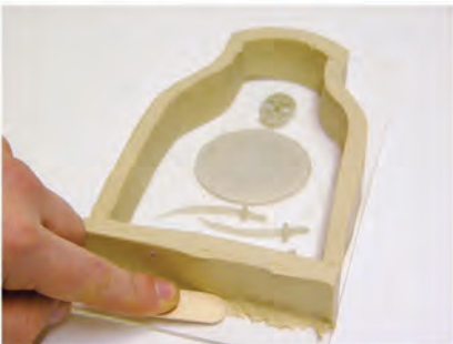
19. Make a clay wall 10mm around sculpture. Press down clay edges to create a seal.
