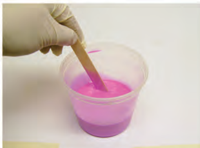
23. When mixed to a uniform colour and swirl free, Pinky is ready to be applied.
