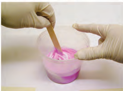
22. Mix thoroughly. Pinky silicone has only 6 mins of worktime.
